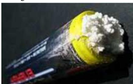
**Fig1. A Leaking Electrochemical Battery**
