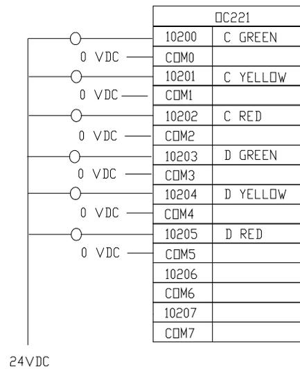
Figure 2.8 Output wiring diagram
