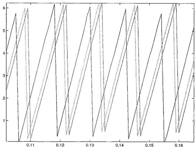
**Figure 4:** Rotor position angles:  $\theta_{sensor}$  (blue),  $\theta_{hat}$  (green),  $\theta_{ctr}$  (red). Experiment #1.
