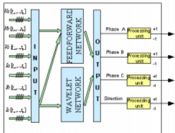
Fig. 4. MLF-DWT relay
