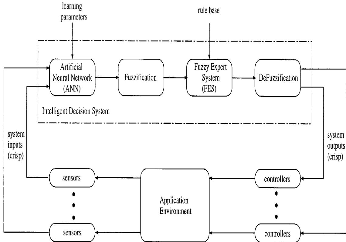
**Figure 5. IDUTC architecture**
