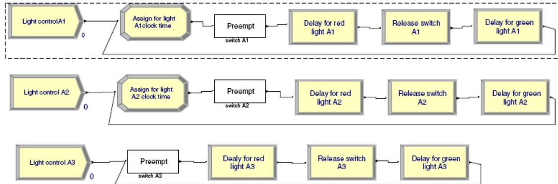
*Figure 3. The simulation flow diagram for Traffic Light A1*
